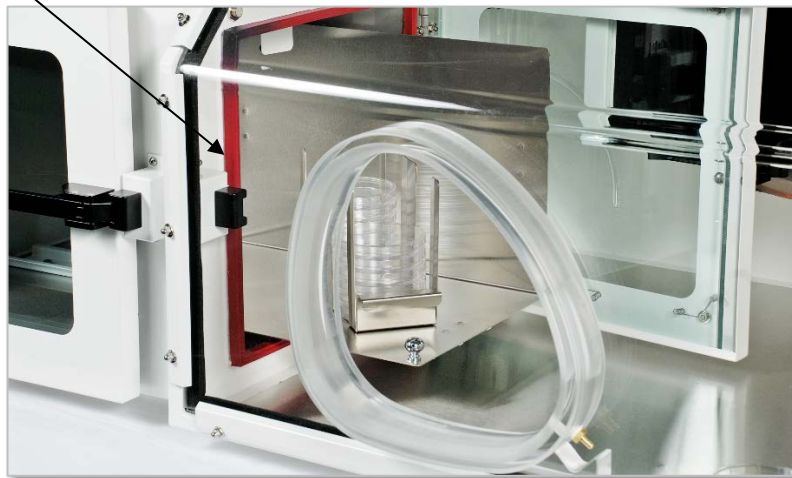
Figure 7: Airlock Inner Door and Sliding Shelf
