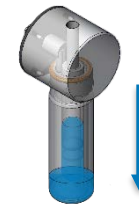
Water in manometer outer bottle forced down
