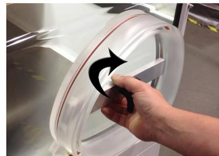
**Figure 21: Securing the Arm Port Doors**
