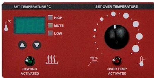
Figure 18: Incubator & OTL Controls
